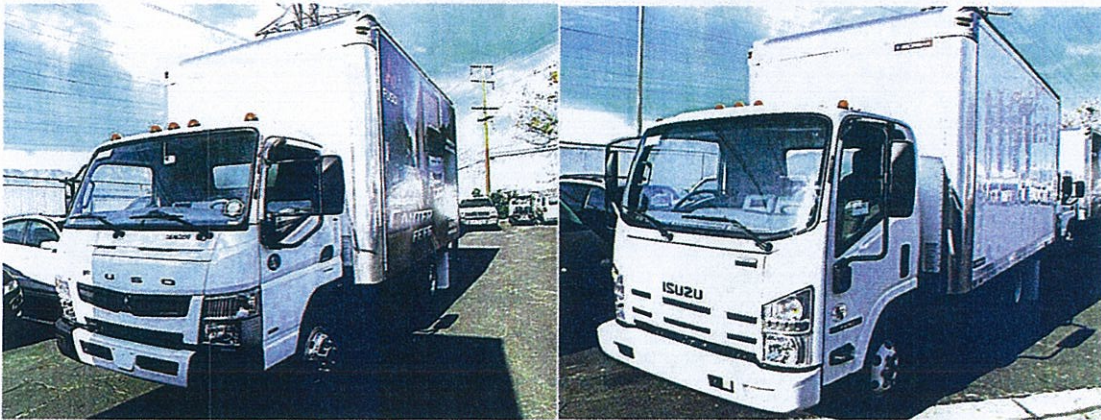
Figure 1: MFTA Fe160 and Isuzu NPR-HD Trucks used in fuel test program without roof fairing.
