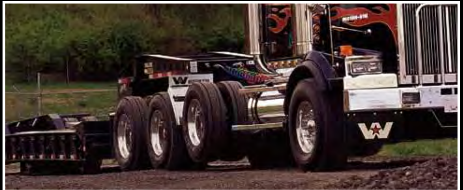
Air-Lift axles help satisfy Bridge Law Requirements.
